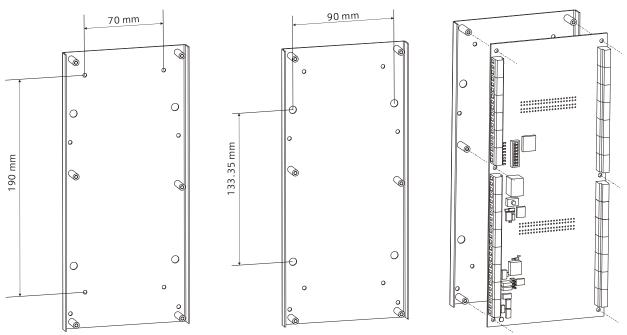
Fig.2 Installation size for wall-mounted
