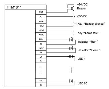
Fig.5 Connection diagram 1
