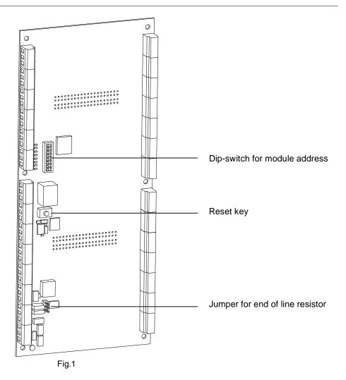
**Dip-switch:** To set FTM1811 FR18-BUS(CAN-Bus) address, digit 1~5 are available for address 1~31, digit 6~8 are reserved.
